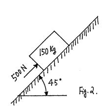
2. A 500-N force acts on a 150-Kg block placed on an inclined plane.
