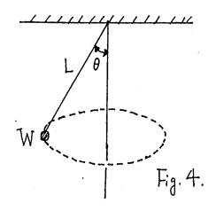
A conical pendulum ball of weight W attached to a cord of length L, as shown in Fig. 4., is revolving in a horizontal circle at a constant speed Vo. Let the angle formed by the cord with the vertical be  $\theta$ . Neglecting the weight of the cord, determine (a) the tension in the cord and (b) the speed Vo, in terms of W, L, and  $\theta$ . (20%)
