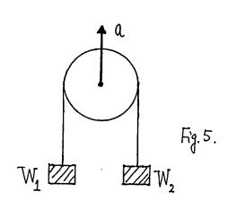
Two weights  $W_1$  and  $W_2$  are hung from a flexible, but inextensible, cord over a frictionless pulley which moves upward with an acceleration a (Fig. 5.). Assuming that  $W_2 > W_1$  and neglecting the rotating inertia of the pulley, derive an expression for the tension in the cord. (15%)
