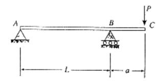
4. A bar of rectangular cross section is loaded and supported as shown in the figure. The distance between supports is L=1.5 m and the height of the bar is h=120 mm. The deflection  $\delta$  at the midpoint is measured as 2.5 mm. What is the maximum normal strain  $\epsilon$  at the 10p and bottom of the bar? (30%)
