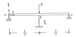
2. For the system as shown, draw the influence line for the internal spring force ( $F_s$ ). Plot numerical values every 0.1L. Assume the flexibility of the spring  $f_s = \frac{L^3}{48EI}$ , and the bending rigidity of the beam EI=constant. (25%)
