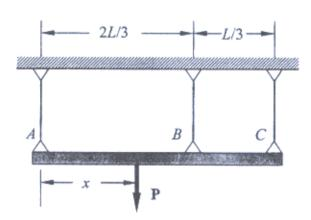
For the cantilever beam ABC, determine the deflection at (a) point B, (b) end C.
