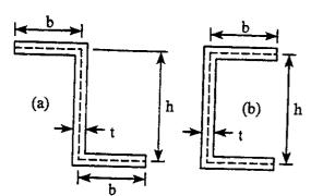
2. Determine the locations of the shear centers S of the (a) Z section and (b) channel section with uniform thickness t? (20%)
