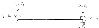
Fig. 2(a): The nodal displacements and forces defined according to the global coordinate system.
