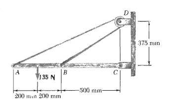
3. (10%) Determine the magnitude of the moment reaction at the beam support (i.e.,  $M_A$ ) for the given loading.
