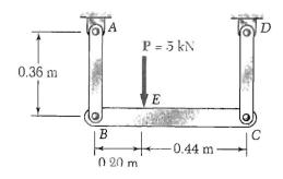
3.(15pts) The solid rod BC has a diameter of 30 mm and is made of an aluminum for which the allowable shearing stress is 25 MPa. Rod AB is hollow and has an outer diameter of 25 mm; it is made of a brass for which the allowable shearing stress is 50 MPa. Determine (a) the largest inner diameter of rod AB for which the factor of safety is the same for each rod, (b) the largest torque that may be applied at A.
