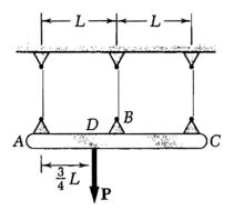
3. (10pts) Draw the shear and bending-moment diagrams for the beam and loading shown.
