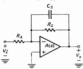
(a) If the op amp is ideal and has an infinite open-loop gain,  $A(s) = \infty$ , find the closed-loop gain, G(s). (5  $\Re$ )
