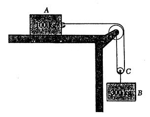
(15%) A 50-kg pulley having a radius of gyration of 0.4 m is connected to two cylinders as shown. Assuming no axle friction, determine the angular acceleration of the pulley and the acceleration of each cylinder.
