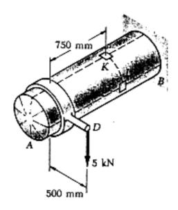
5. (25pts) Determine the reaction at the roller support and draw the bending moment diagram for the beam and loading shown.
