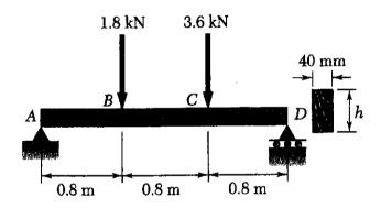
6.(20pts) For the beam and loading shown, determine the deflection at the midpoint D. Use E = 200 GPa and  $I = 6.87 \times 10^{-6}$  m<sup>4</sup>.
