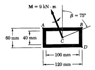
5.(20pts) For the beam and loading shown, design the cross section of the beam, knowing that the grade of the timber used has an allowable normal stress of 12 MPa.
