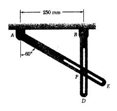
8. The motion of pin P is guided by slots cut in rods AE and BD. Knowing that the rods rotate with the constant angular velocities  $\omega_A = 4$  rad/s clockwise and  $\omega_B = 5$  rad/s clockwise. For the position shown, determine (a) the magnitude of the velocity of pin P and (b) the magnitude of the acceleration of pin P.
