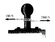
3. A rope is wrapped two full turns around a short column as shown. The tension in the rope is 7500 N, and a force of 150 N has to apply on its free end in order to just keep rope from slipping to the right. (a) Calculate the coefficient of friction between the rope and the column. (b) Calculate the tension in the rope that would be resisted by the 150-N force if the rope were wrapped three full turns around the column.
