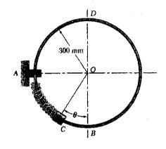
6. A circular rod is supported in a vertical plane by a bracket at A. Attached to the bracket and loosely wound around the rod is a spring of constant k = 40 N/m and undeformed length equal to the arc of circle AB. A 200-g collar C, not attached to the spring, can slide without friction along the rod. Knowing that the collar is released from rest when  $\theta = 30^{\circ}$ , determine (a) the maximum height above point B reached by the collar and (b) the maximum velocity of the collar.
