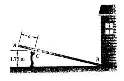
1. A worker is raising a 9.2-m-long ladder of mass 53 kg as shown. Knowing that a = 1.8 m and that the force exerted by the worker is perpendicular to the ladder, calculate (a) the magnitude of the force exerted by the worker and (b) the magnitude of the reaction at B.
