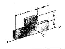
4. Denoting the mass of the thin plate by m, determine its mass moment of inertia with respect to (a) the axis AA' and (b) the centroidal axis CC' that is perpendicular to the plane of the plate.
