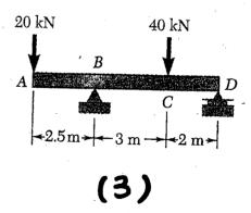
Draw the shear and bending-moment diagrams for the beam and loading shown.
