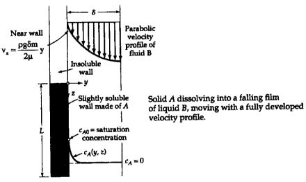
It is assumed that the velocity  $v_z$  of liquid B depends only on y for z > 0. In addition, the wall is made of a species A that is <u>slightly soluble</u> in B, thus for short distances downstream, species A will not diffuse very far into the falling film. That is, A will be present only in a very thin boundary layer near the solid surface. Therefore, the diffusing A molecules will experience a velocity distribution that is characteristic of the falling film right next to the wall, y = 0.
