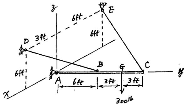
3. 試求 B 真重直及水平位移。設二桿  $A_1 = 2 \text{ in}^2$ ,  $A_2 = 3.5 \text{ in}^2$ ,  $E = 10.6 \times 10^3 \text{ ksi}$ .
