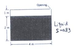
what will be the maximum pressure intensity in the tank during acceleration?
