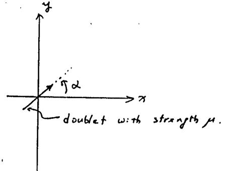
(b) If the doublet of problem (a) is located near an infinitely long wall, what will be the expressions for the stream as well as the potential functions? The coordinate system is shown below.
