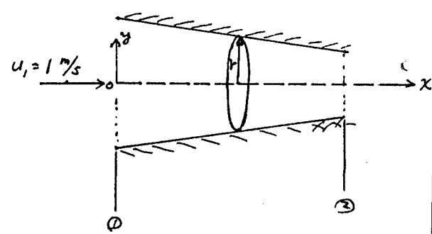
the volume flow rate decreases linearly with time from the above value at  $t = 0$  to zero at  $t = 10$  seconds. Find the acceleration  $a$  in the nozzle during the interval  $0 \leq t \leq 10$  sec. (Assume one dimensional flow.)
