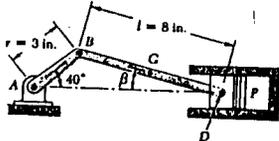
Crank AB of the engine system has a constant clockwise angular velocity 2000 rpm. For the crank position shown, determine the angular acceleration of the connecting rod BD and the acceleration of point D. (20%)
