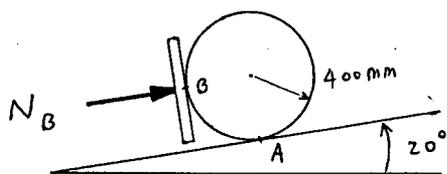
A 100 kg steel pipe of radius 400 mm is pushed up the  $20^\circ$  incline at constant velocity as shown
