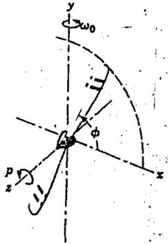
The two-bladed airplane propeller has a constant rotational speed  $p$  about its shaft axis  $z$  and a moment of inertia  $I$  about this same axis. The airplane is turning
