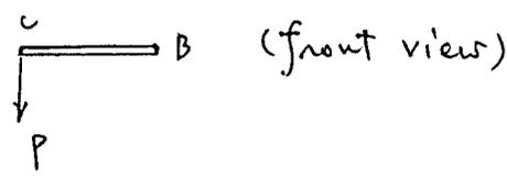
The structure shown consists of a round tube, section properties  $EI$ ,  $GJ$ , length  $L$ , in a horizontal plane. The free end supports a load  $P$ . Please find the vertical displacement of the point  $C$ . (20%)
