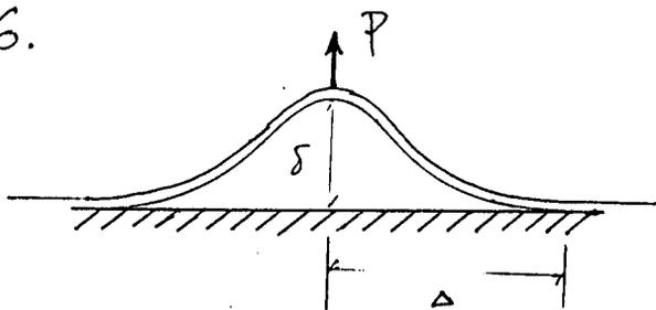
An infinite beam is rested on a rigid foundation and pulled by a concentrate force
