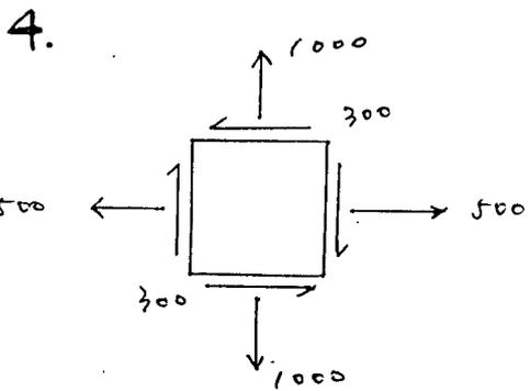
The element shown here is subjected to two set of stresses at the same time. Find, by using Mohr's circle, the magnitudes of the normal and shearing stresses on
