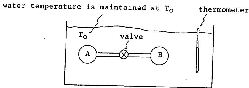
Joule's experiment: When valve is open, gas in A expands into vacuum B. Bulbs A and B have the same volume.
