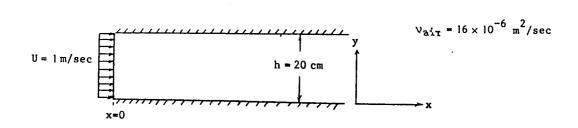
Assume that boundary layer developed on the wall from x=0 to 1m is laminar, where the boundary layer thickness,  $\delta$ , the displacement thickness,  $\delta^*$ , and the momentum thickness,  $\theta$ , are expressed as follows.
