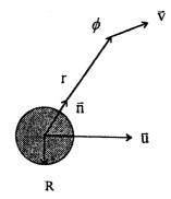
r: distance from center of cylinder to a position in flow field.
