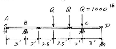
(25%) 2. Determine the horizontal and vertical components of force that the pins at A, B, and C exert on their connecting members.
