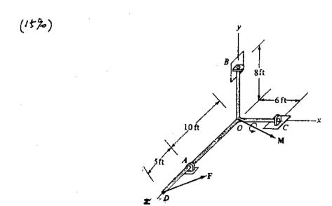
2. Determine the forces acting on each member of the frame in the figure
