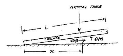
A flat plate is hinged at one side to s smooth floor, as shown, and held at a small angle  $\theta_o$  ( $\theta_o \ll 1$ ) relative to the floor. The entire system is submerged in a liquid of constant density  $\rho$  At t = 0, a vertical force is applied and adjusted continually so that the rate of decrease of the plate angle  $\theta$  remains constant at a value  $\omega$ :
