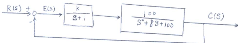
It is required to select a suitable value of  $K$  so that the steady state tracking error for a unit step input is less than 0.1. Is it possible to find such a  $K$  value? Justify your answer.
