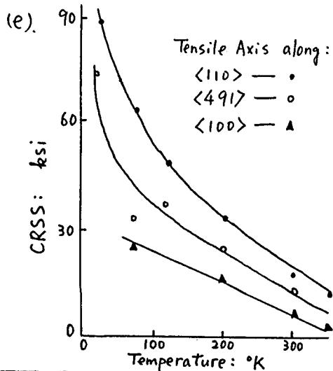
The CRSS of  $\langle 110 \rangle \langle 111 \rangle$  slip as a function of test temperature and tensile axis direction is shown in the figure for pure molybdenum. The crystal structure of molybdenum is bcc. The data in the figure do not fall on a single curve, whereas those for fcc materials do fall on a single curve. Why? (7%)
