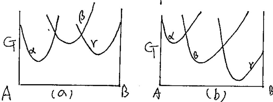
Illustrate the stable phases through the composition range for Figs. (a) and (b). (10%).
