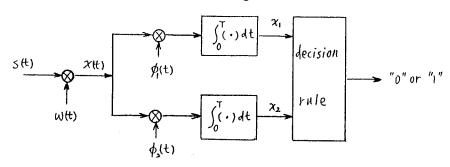
w(t) represents a white Gaussian noise with power spectral density  $N_0/2$ .  $s(t) = s_1(t)$  if "0" is sent,  $s(t) = s_2(t)$  if "1" is sent. The waveforms of  $s_1(t)$  and  $s_2(t)$  are given below.
