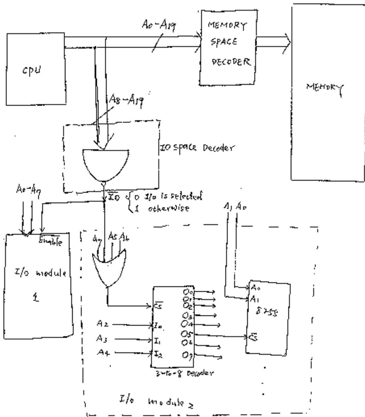
Note: CS is the chip select, 0 means enable the chip to work, 1 otherwise
