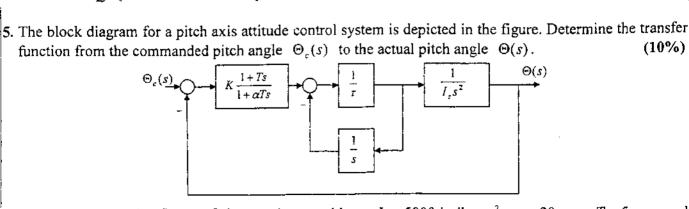
6. Suppose that in the figure of the previous problem,  $I_z = 5000 \text{ in-lb-sec}^2$ ,  $\tau = 20 \text{ sec}$ , T = 5 sec, and K = 200. Determine the range of  $\alpha$  so that the closed-loop system is stable. (10%)
