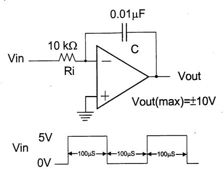
6. Plot the output voltage waveforms, Vout, of the following figures (a), (b), (c), and (d), respectively. Note: the diode forward voltage V<sub>F</sub>=0.7V. (10%)
