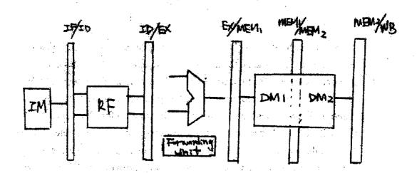
2. For the above pipelined processor, come up with the behavioral code for the logic of the forwarding unit assuming MIPS-like ISA is used. State you assumptions if any. (20%)
