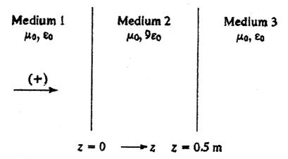
6. For the system shown below, find the input impedance of the line and the time-average power delivered to the load. (20 分)
