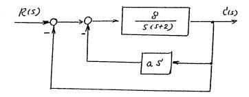
3. The characteristic equation of a servo control system is given as:  $s^3 + 3 k s^2 + (k+2) s + 4 = 0$ Determine the range of value "k" for the system to be stable?
