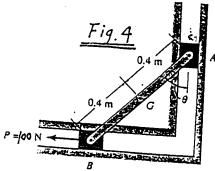
4. The 10-kg rod shown in Fig.4 is constrained so that its ends move along the grooved slots. The rod is initially at rest when  $\theta=0^{\circ}$ . If the slider block at B is acted upon by a horizontal force P=100 N, determine the angular velocity of the rod at the instant  $\theta=4.5^{\circ}$ . Neglect the mass of blocks A and B. (25%)
