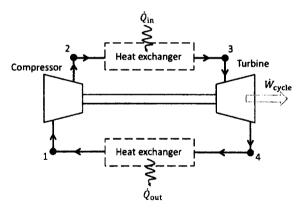
5. (a). A schematic diagram of an air-standard gas turbine is shown above. Draw the p-v diagram of air-standard ideal Brayton cycle. Mark points 1, 2, 3, and 4. Specify the cycle direction in the diagram. (10%)
