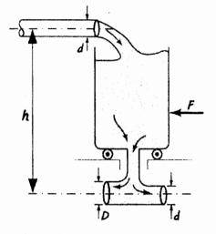
Water flows steadily into and out of a tank that sits on frictionless wheels as shown above. Suppose that the inlet pipe is at a height h above the two discharge pipes, but is at a negligible height over the water surface inside the tank. (Assuming  $D, d \ll h$ , it is appropriate to neglect the distance between the centerlines of the left and right discharge pipes when  $D \neq d$ .) Let us also neglect viscous losses.
