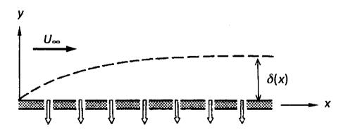
Using the approximate integral method and assuming similarity of the velocity profile, i.e. that  $u/U_{\infty}=f(y/\delta)$  where f is not a function of x, find a relation between the frictional coefficient,  $c_f=2\tau_w/\rho U_{\infty}^2$ , and the quantities V,  $U_{\infty}$ ,  $d\delta/dx$ , and  $\alpha$  where  $\alpha$  is the profile parameter
