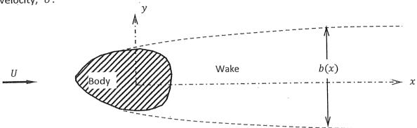
The surveys are made at *x* locations sufficiently far downstream of the body so that the pressure across the wake is the same as the ambient pressure in the fluid far from the body. They indicate that, to a first approximation, the velocity in the wake varies with lateral position, *y*, according to
