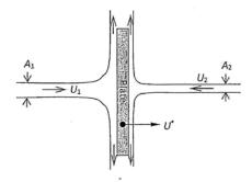
The jets are uniform far from the plate and have unequal velocities,  $U_1$  and  $U_2$ , and cross-sectional areas,  $A_1$  and  $A_2$ , as shown. The deflected jets leave the plate with zero component of horizontal velocity <u>relative</u> to the plate. If the plate is free to move horizontally (while remaining vertical) at what steady velocity,  $U^*$ , will it travel? Assume that the pressure in the jets far from the plate is atmospheric. Neglect any effects of gravity.
