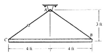
4. A stiff bend rod is dropped so that end A strikes a heavy table D. If the impact is plastic and there is no sliding at A, what is the postimpact speed of end B? The rod weighs per unit length 3 kg/m. (15%)
