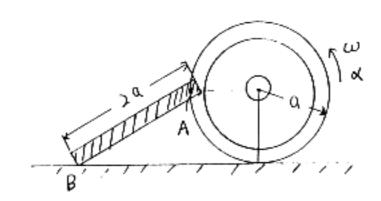
2. The rod of length L and mass m is released from the rest when  $\alpha = 0^{\circ}$ . If the coefficient of static friction at A is  $\mu$ , determine as a function of  $\alpha$  the forces which are exerted on the ledge at A as it falls downward.
