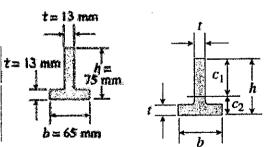
$c_1 = 50.2 \text{ mm}, c_2 = 24.8 \text{ mm}, I = 850195 \text{ mm}^4$
