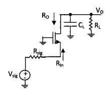
6. The following figure shows an ideal voltage amplifier with a gain of -1000 V/V. (a) Use Miller's theorem to find the input capacitance ( $C_{in}$ ) of the amplifier. (10%) (b) Find the 3-dB frequency  $f_H$  (Hz) of the transfer function ( $V_O/V_{sig}$ ). (5%)
