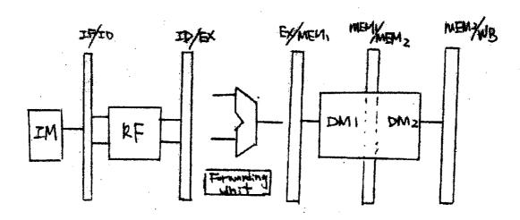
2. For the above pipelined processor, come up with the behavioral code for the logic of the forwarding unit assuming MIPS-like ISA is used. State you assumptions if any. (20%)
