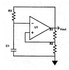
2. Given the following high pass filter circuit. Let Let  $R_1 = R_2 = 10 \text{K} \Omega$ ,  $C_1 = 0.1 \mu\text{f}$  and  $C_2 = 0.2 \mu\text{f}$ . (a) Find the cut-off frequency. (10%) (b) Give the transfer function. (10%) (c) Sketch its Bode-plot with respect to the input and output voltages. (10%) (d) Give the Q factor. (5%)
