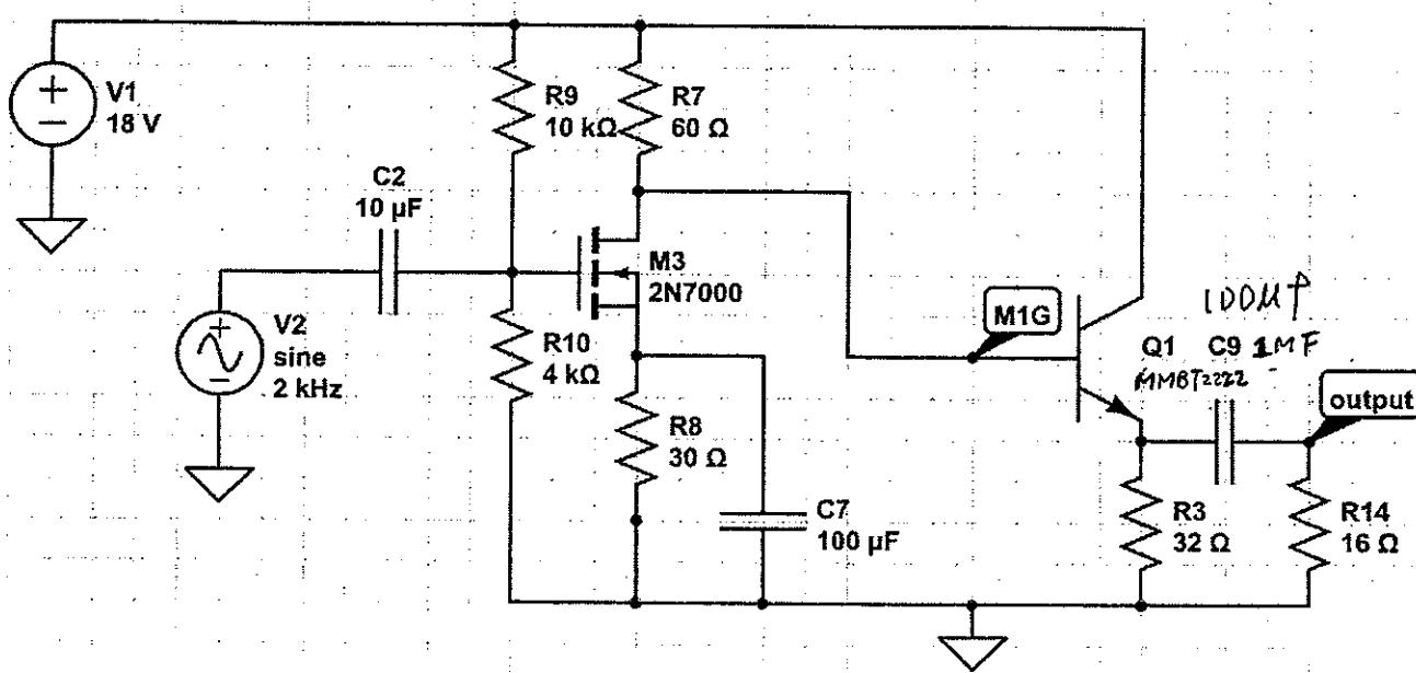
2. Given the following bandpass filter circuit. Give the magnitude frequency response in the range from 50Hz to 5KHz. (30%) Show all details.
