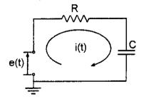
resistance R and a capacitor with capacitance C. If the input voltage is
